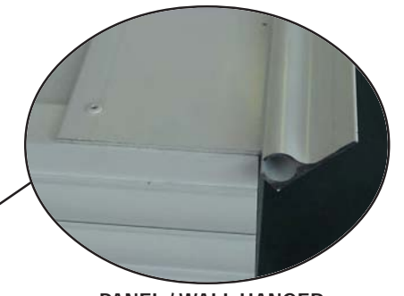
PANEL / WALL HANGER Structural support designed to allow for expansion and maintain a water tight seal when lagged onto the second floor sill plate, rafter tails or studs depending on the application. Adjustable up to 5/12 roof pitch.
